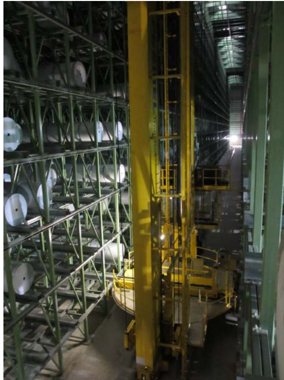
Figure 3, TransRoll stacker crane sorting rolls at APRIL Fine Paper's Xinhui mill.
