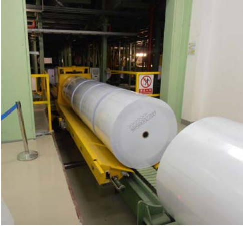
Figure 5, Gentle multi roll handling by TransRoll channel vehicle at the Intermediate Roll Storage (IRS) in-feed.
