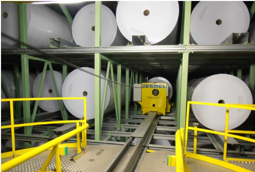
Figure 7, TransRoll vehicle fetching rolls according the orders from the storage to be delivered forward to wrapping and shipping.
