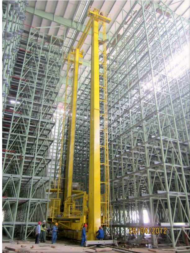
Figure 8, There are motors only in the TR- vehicle and stacker crane, which technology resembles roughly vertically turned overhead crane.
