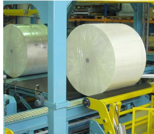
These two Pesimal packaging lines include the automated change of a stretch film roll as the film runs out. This function changes the empty film roll to a new one automatically without presence of an operator and continues the roll wrapping. Maximum pre-loading capacity of 8 pcs of 80 kg film rolls is 640 kg in total in one loading. The film roll storage magazine can be loaded when the wrapping function is running.
