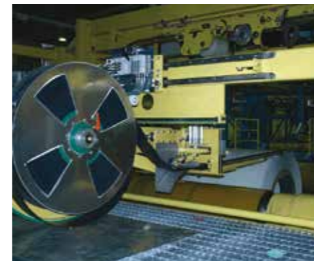
Integrated edge protection for sharp edge and sensitive materials
