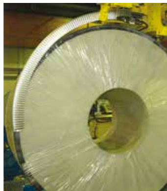
Automated outer edge protection
