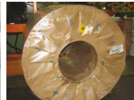
Manually packed coil (VCI paper) - VCI evaporates because of air circulation.
