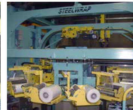
Automated PE film changing device with 12 film rolls
