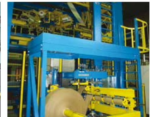
Automatic material winder winds correct sized rolls for wrapping
