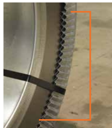
Manually inserted outer edge protection (overlapping, 30% more waste)
