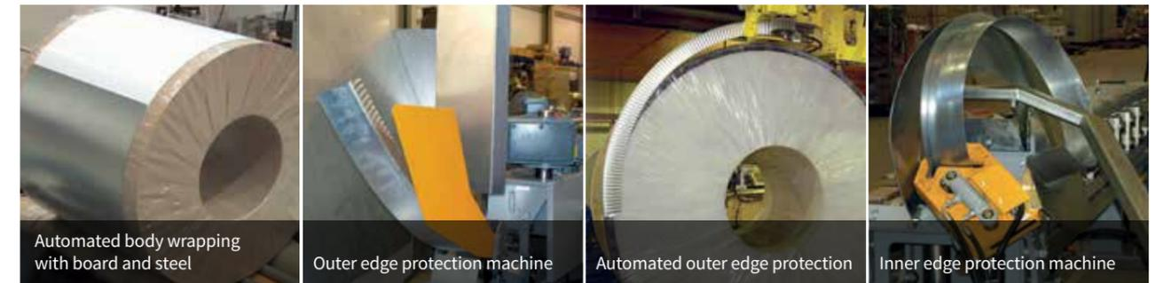
Automated body wrapping with board and steel
