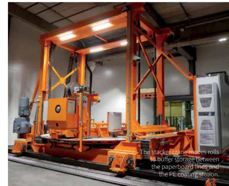
The stacker crane moves rolls to buffer storage between the paperboard lines and the PE coating station.
