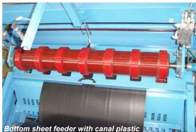
*Bottom sheet feeder with canal plastic*
