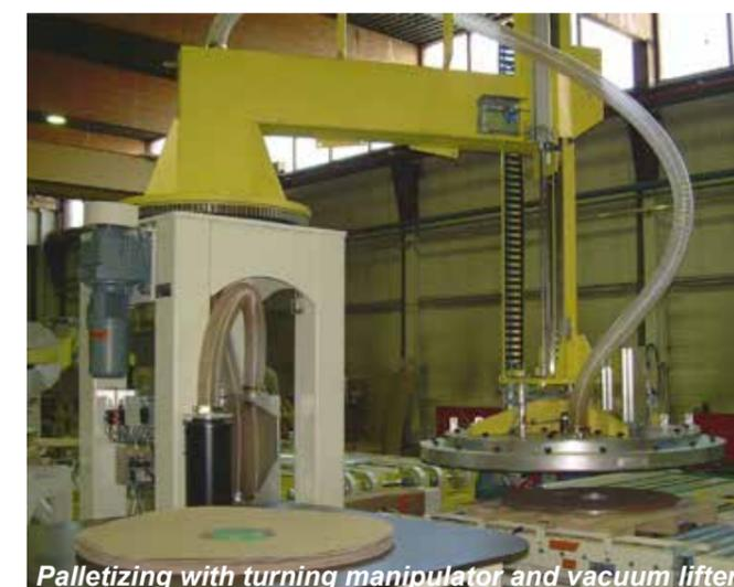
Palletizing with turning manipulator and vacuum lifter
