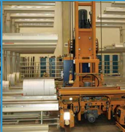
Narrow roll handling for packing is done by sorting carriage.
