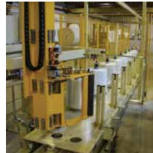
*Automated film roll changing magazine allows 24 hours continuous operations.*
