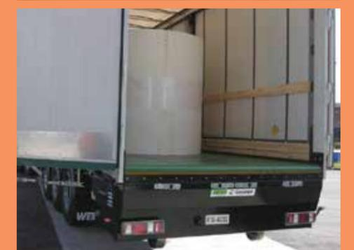
*Automated truck loading or unloading procedure takes only five minutes and is done without any clamb truck handling.*
