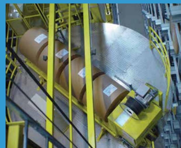
*Load forming and sorting is done automatically by TransRoll® stacker crane.*
