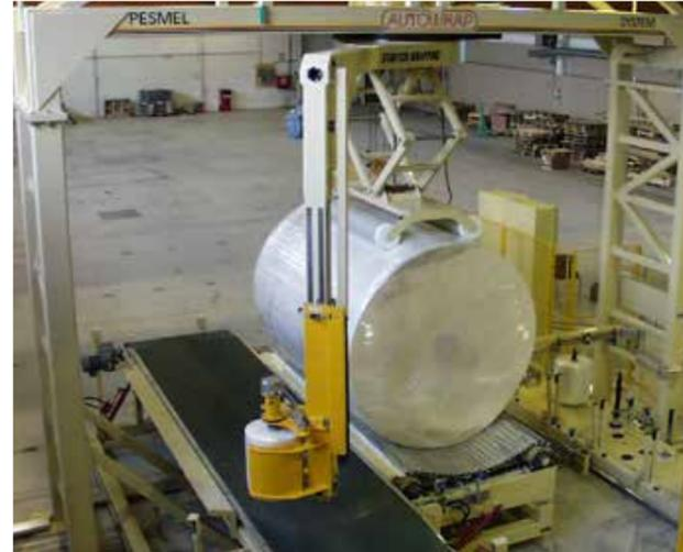
*High capacity tissue packing system with patented roll turning cradle.*
