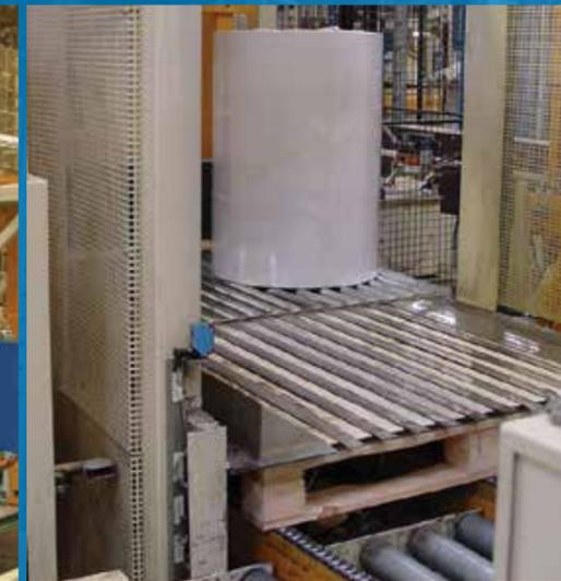
Plate palletizer for vertical palletizing can be used for single or multi-stacks.
