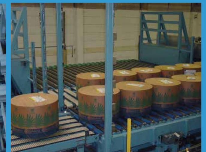
*Sea cassette load forming and loading is done automatically in six minutes.*
