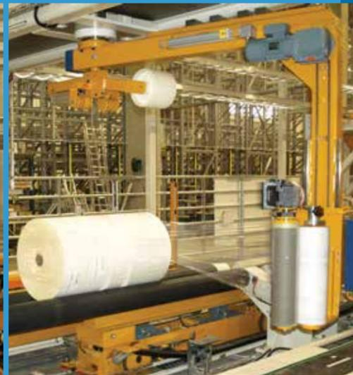
Automated axial wrapping is tying the rolls into a stack.
