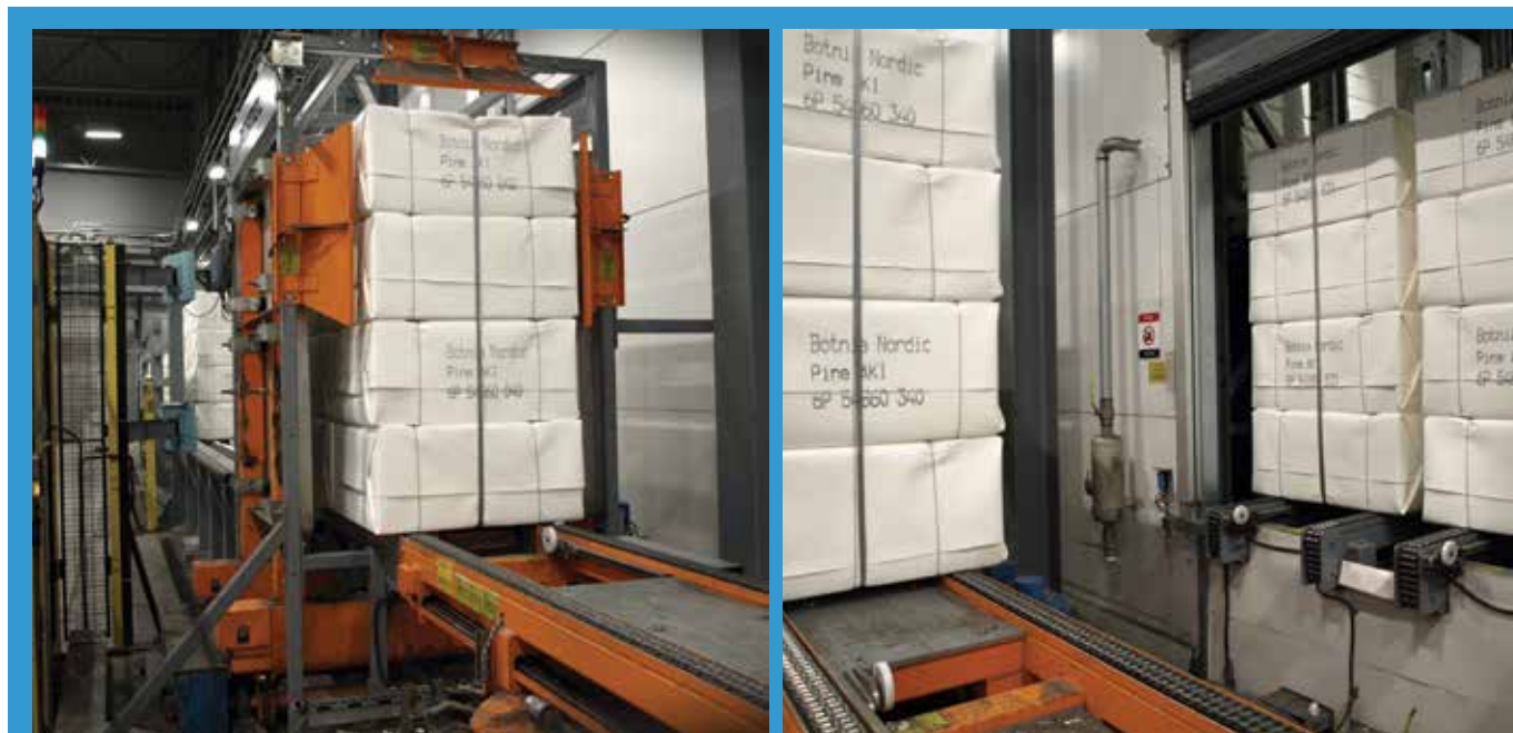
TransBale handles the pulp bales from the bottom.
