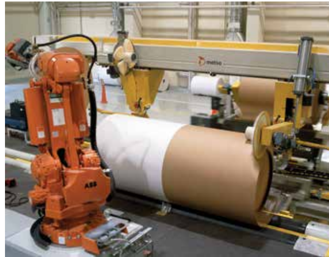
Over-lap wrapping method offers a cost efficient and space saving solution to wrap wide rolls.
