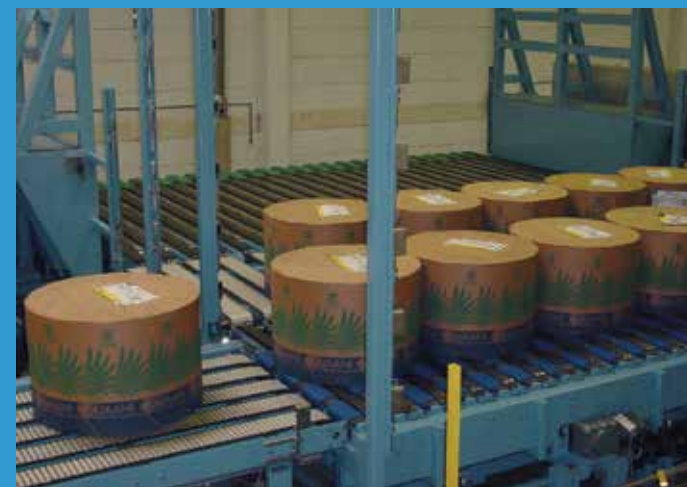
Sea cassette load forming and loading is done automatically in six minutes.
