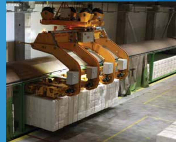
With automatic loading a train with 22 cars carrying 1 400 tons of pulp can be loaded in three hours.
