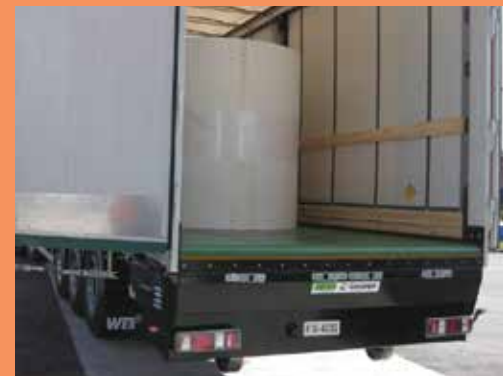
Automated truck loading or unloading procedure takes only five minutes and is done without any clamb truck handling.
